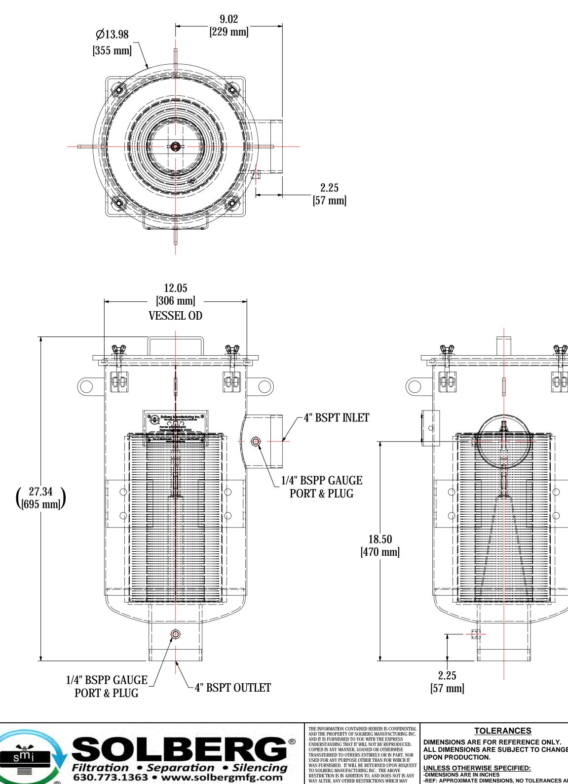
UNLESS OTHERWISE SPECIFIED: -DIMENSIONS ARE IN INCHES -REF: APPROXIMATE DIMENSIONS, NO TOLERANCES AF -FINISH: BREAK EDGES TO .005-.020 RADIUS/CHAMFER
